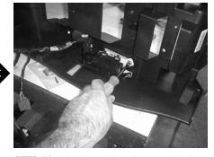
**STEP 14:** With the outside wall removed, lay the console on its side. Using a 7mm socket, unsecured and remove the wiring harness.
